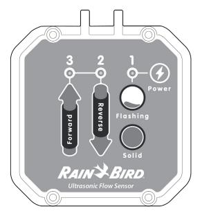
The status of your UFS Series Ultrasonic Flow Sensor can be determined by the LED lights on the upper body, or tested at the connection point of the controller. The sensor is essentially a 15 Ohm switch with a  $600 \mu A$  leakage current. With no flow running, the sensor will appear to the controller input as a small current load. When flow is running, it appears a quick series of 5 millisecond short circuits.
