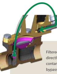
Filtered water flows directly through the contamination-proof bypass tube.
