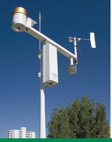
Weather stations provide a wide range of local weather information on a daily basis that can be used to manage irrigation at a site or across a number of sites.
