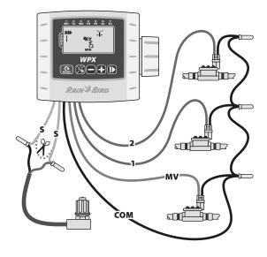
NOTE: The WPX can be mounted on a DC latching solenoid using the included solenoid bracket, or on a wall using the optional wall-mount bracket (Model: 9VMOUNT).
