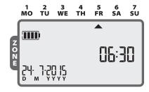
In **AUTO RUN** mode, the WPX will irrigate each zone per its programmed schedule. If any zones are scheduled to run at the same time and day, your controller will place those zones in a queue and irrigate one valve at a time, starting with the lowered number zone first.
