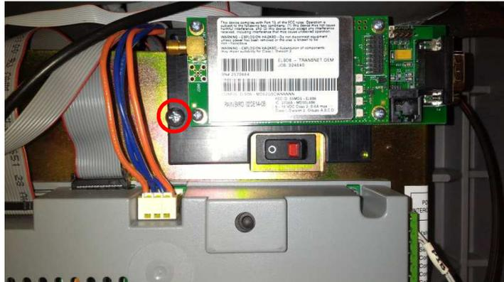
5. Secure the radio/modem in place using a drill to drive the two 3/16 6-20 thread self-tapping screws into the PAR+ES metal bracket through the plastic mount plate on either side of the power switch. Place the paper slip over the top of the PIB to prevent metal shavings from entering the PIB while drilling.
