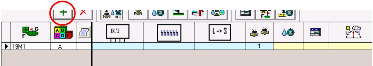
4. Select the ICI wire path where the IC-OUT is connected and enter the IC-OUT address noted from the barcode label. In the example below, the IC-OUT is connected to wire path 1 and its address is 0FE93F:
