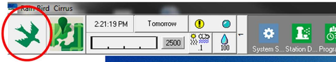
3. If the software version is less than **8.1.0**, (as viewed below) contact your Rain Bird distributor for options to acquire new software. Rain Bird distributors and / or Rain Bird GSP can assist with software updates.
