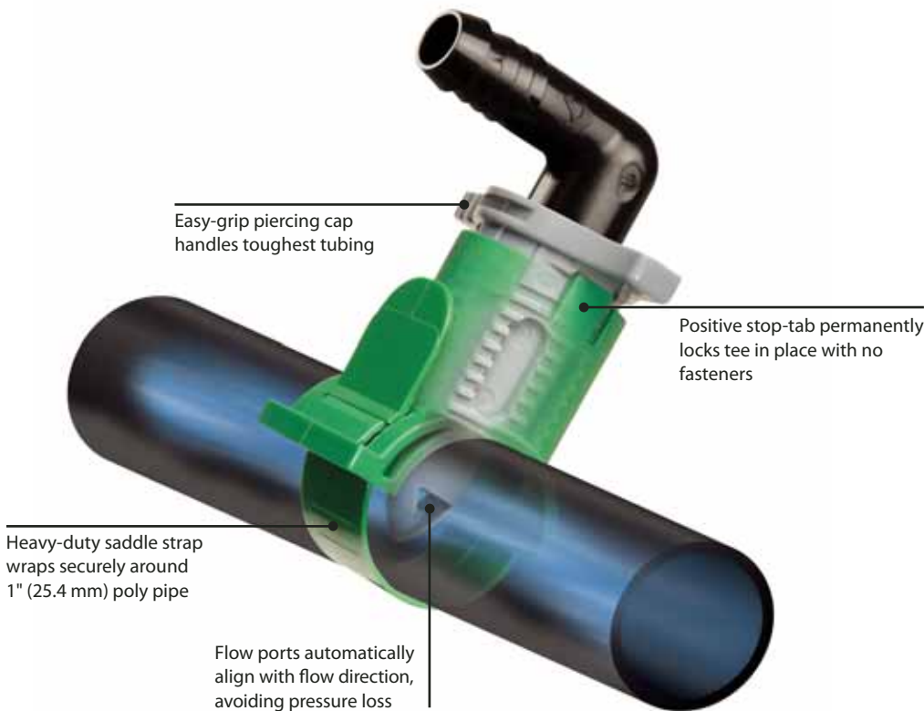
Wrap the ratchet locking saddle around pipe and tighten securely
