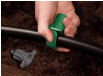
Wrap the ratchet locking saddle around pipe and tighten securely
