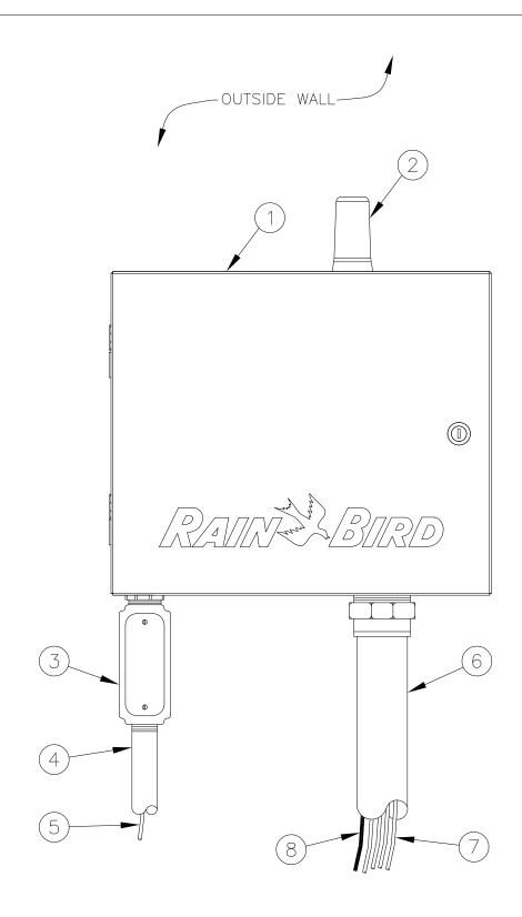
IQ ESP-LXMEF SATELLITE CONTROLLER WITH FLOW SMART MODULE
