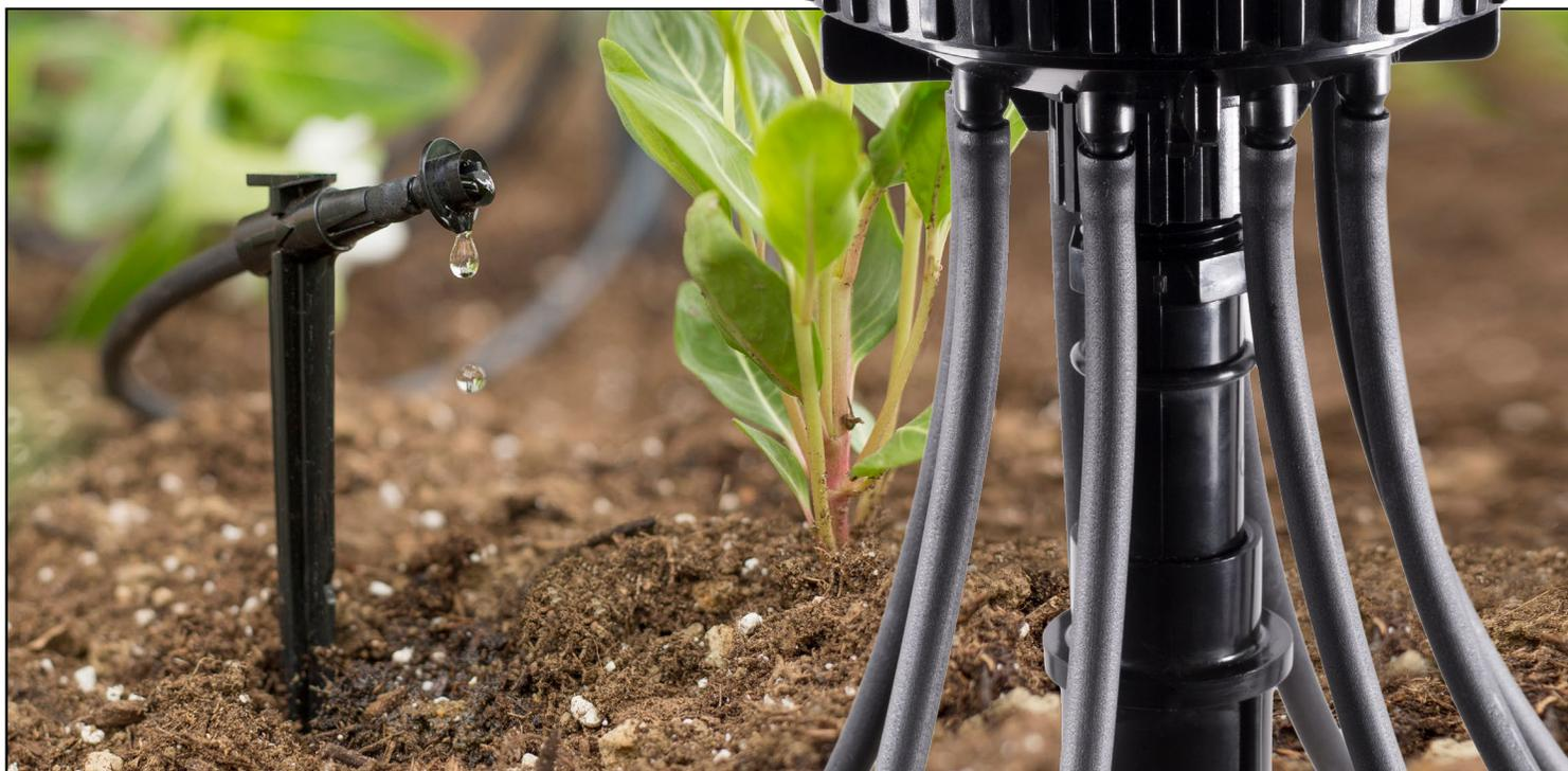
A low volume irrigation system typically applies water slowly, at low pressure, at or near the root zones of the plant material. Whether referred to as drip, micro-irrigation, or low volume, these systems feature emission devices that apply water in gallons per hour (GPH) as opposed to the gallons per minute (GPM) of a conventional overhead spray irrigation system.
