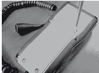
Unscrew the field transmitter back plane.
