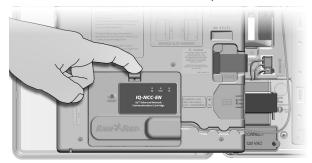
3 Locate (or remove) the small knockout on the bottom of the controller cabinet and run the wifi adapter's power connector through the hole and into the cabinet.
