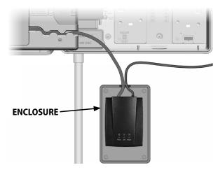
Plug the wifi adapter cable and power connector into the wifi adapter unit and secure the enclosure lid.
