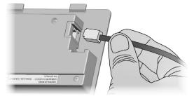
5 Replace the cartridge and route the wifi adapter cable through the cable channel.
