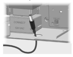
4 Plug the wifi adapter cable into the connection jack on the back-side of the NCC cartridge.
