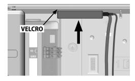
**NOTE:** Do not place wifi adapter directly touching the controller connection module or any adjacent field wiring modules.
