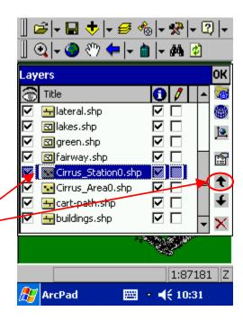
j. Next, adjust the layer properties. Tap the layer that will be adjusted. Start with the Cirrus\_Station0 layer, as it needs to be set first and hyperlinked with the FREEDOM-Pad activation program. Tap the **Properties** icon.
