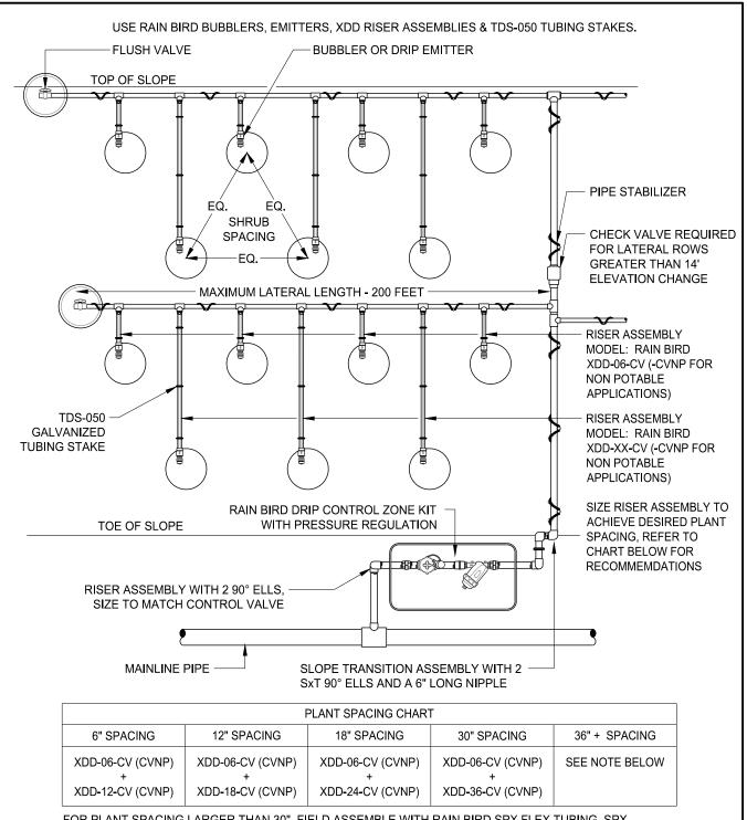
FOR PLANT SPACING LARGER THAN 30", FIELD ASSEMBLE WITH RAIN BIRD SPX FLEX TUBING, SPX FITTINGS, XT050CV (OR XT050CVNP) CHECK VALVE, AND TDS-050 GALVANIZED STAKES
