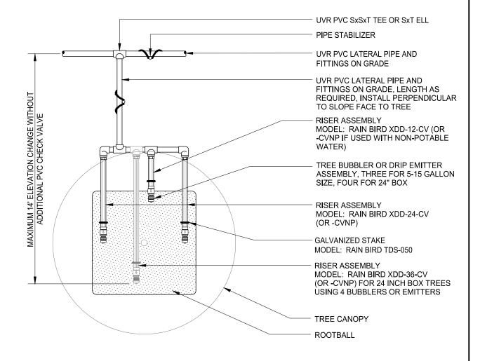
LARGER TREES WITH REQUIRE ADDITIONAL BUBBLERS / EMITTERS EQUALLY SPACED AROUND THE PERIMETER OF THE TREE ROOTBALL
