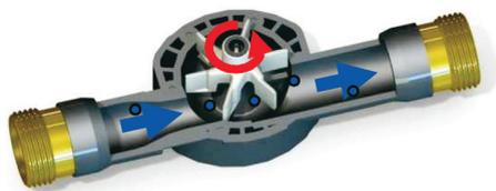
A low friction pivot bearing supports the floating impeller at low flow rates while a thrust bearing provides the support at high flow rates.
