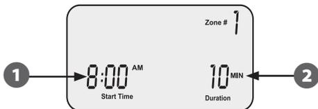
**NOTE:** The STP Plus Controller is designed to prevent any two zones from watering at the same time. This feature is called “Program Stacking”. If more than one zone is scheduled to irrigate at the same time, the next zone will begin irrigating when the previous zone has finished.
