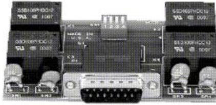
The number of stations can be increased from 4 to 16 in 4 station increments with modules that plug into the rear of the panel. The modules are interchangeable and can be inserted into any module position. Insert a module into connector: #1 to add stations 5 through 8 #2 to add stations 9 through 12 #3 to add stations 13 through 16
