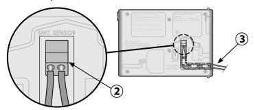
**3** Route the two wires through the provided channel and out through one of the knockouts, located in the bottom of the controller cabinet.
