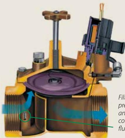
*Filter location prevents clogging and water continuously flushes screen.*
