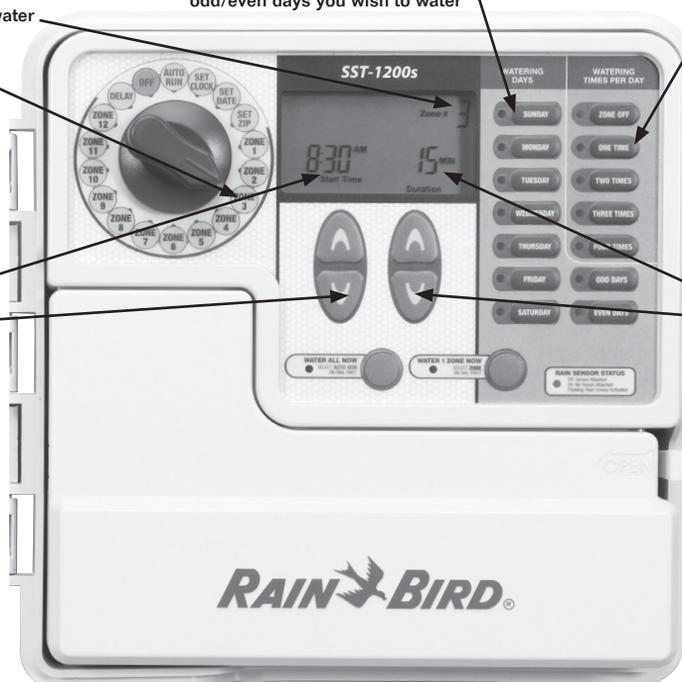
**STOP IMPORTANT:** Reset dial to Auto Run after making any adjustments to the programming
