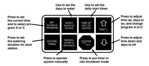
If you're already familiar with this Rain Bird timer, here's a quick guide to what each key does when programming the PC-200 series. For step by step explanations, turn to the following pages. **Note:** use the ARROW keys to adjust any of the following func-
