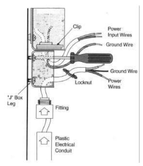
The illustrated "side view" shows how the controller, "J" box, conduit and fitting are used for outdoor installations.
