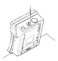
**4.** Slide the controller down over the mounting bracket until lower mounting hole "D" aligns with the hole in the back of the terminal strip compartment. You may want to wait until after you have cut your wire conduits to length before driving the last mounting screw through the aligned holes to secure the controller to the wall or stud.
