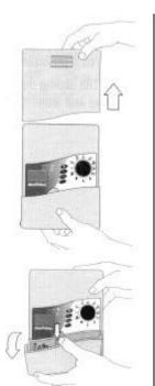
3. Place a flat blade screwdriver in the groove of the knockout labeled "A" in the illustration. With the palm of your hand, strike the end of the screwdriver handle to punch in one side of the knockout. Repeat the process on the other edge of the knockout and remove it. One knockout hole is sized for 3/4" conduit. If the size and number of valve wires require more than 3/4" conduit, punch out the second knockout for 1 " conduit instead.
