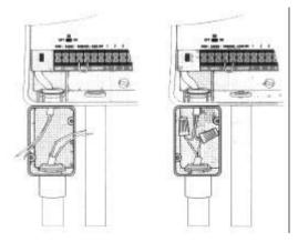
**4.** Carefully coil or bend the wires to fit them and their connectors into the junction box. Reattach the cover to the junction box.
