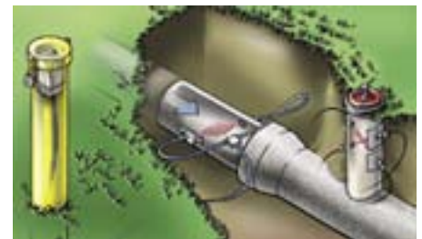
Figure 4. Standard ultrasonic installation. Note that these meters can be installed in a remote favorable location with good hydraulic characteristics.
