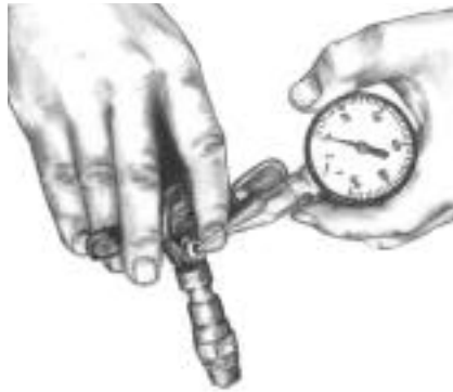
FIGURE 3 Pitot tube shown properly inserted into sprinkler nozzle. (Approx. 1/8" out from nozzle opening)
