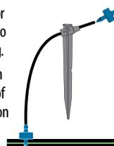
Connect a spiked emitter (on a stake) to drip tubing via a barb connector and 6mm tubing
