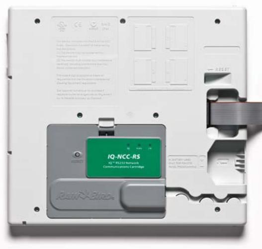
LX Series Cartridge Panel with IQ-NCC-RS Cartridge Installed
