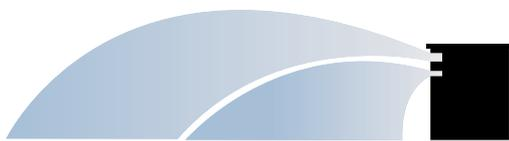
U-Series nozzles offer better, more uniform water distribution. Water flowing from both orifices combines to form a continuous water stream. Eliminates gaps for more uniform coverage throughout the entire watering area
