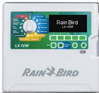
ESP-LXIVM Two-Wire Controller with Smart Valve Technology
