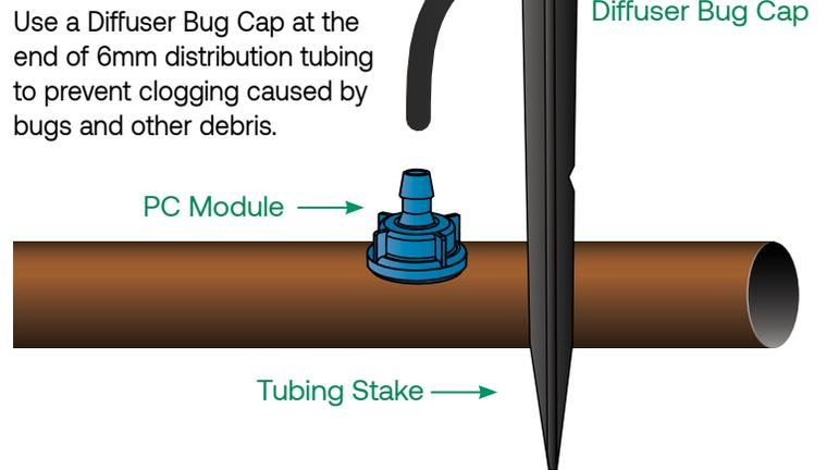
Use a Diffuser Bug Cap at the end of 6mm distribution tubing to prevent clogging caused by bugs and other debris.
