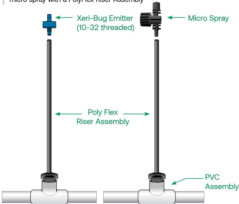
Use an Easy Fit Tee and Female Adapter, to attach a PolyFlex riser with 10-32 thread emitter to drip tubing.
