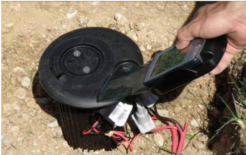
The secondary address label can also be placed on an “as built” plan, an individual hole view, or on field drawings that show the location of the rotor relative to other rotors and hole features. This will also allow the label to be scanned after installation.
