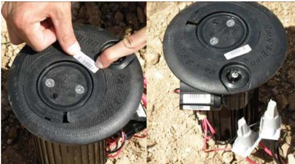
In addition, the label can be scanned prior to the rotor being backfilled using a Rain Bird scanner.
