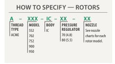
For exact combinations of Rotors (Nozzles and Pressure Regulator), see pages 4–17 for correct model.
