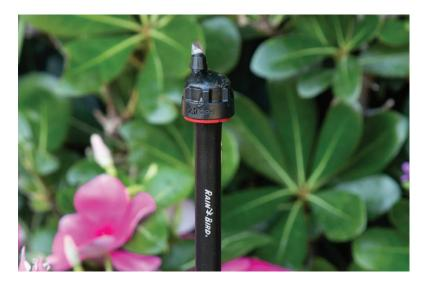
**Pressure Compensating:** Xeri-Bug<sup>™</sup> Emitters with Check Valve maintain a consistent flow rate from 15 to 50 psi (1.0 to 3.5 bar)
